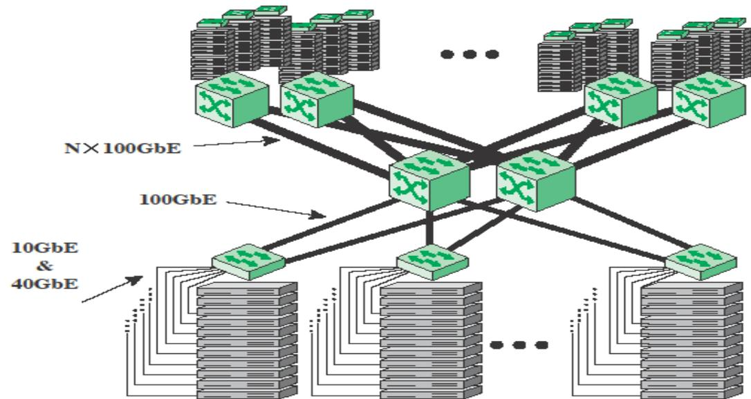
**Figure 16.8 Example 100-Gbps Ethernet Configuration for Massive Blade Server Site**
