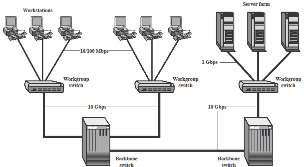
Figure 16.6 Example 10 Gigabit Ethernet Configuration
