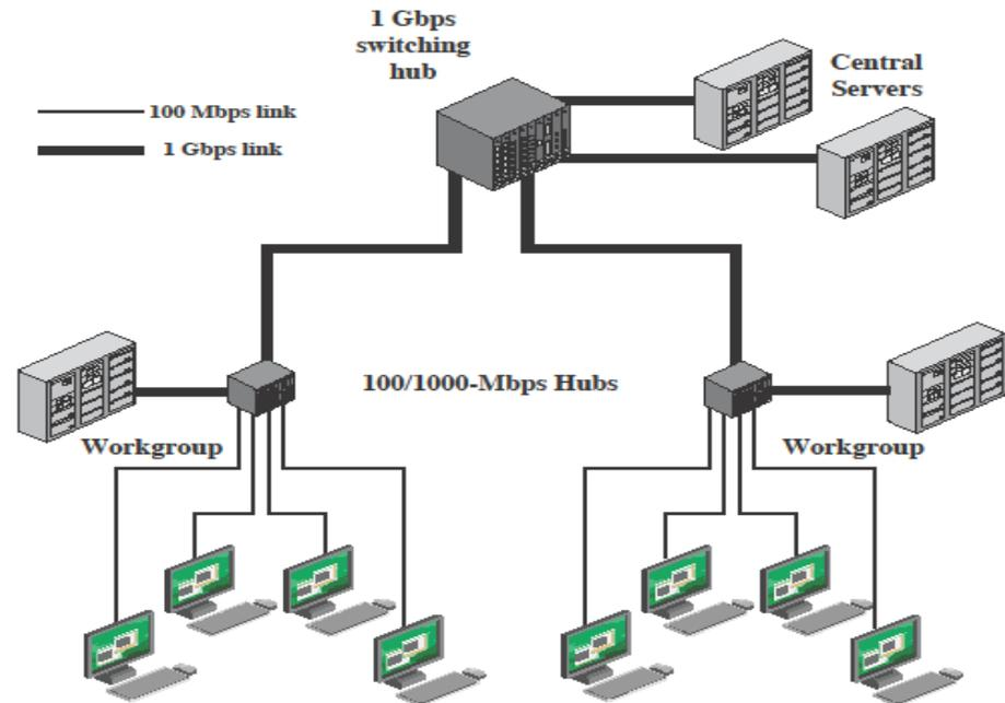
Figure 16.4 Example Gigabit Ethernet Configuration
