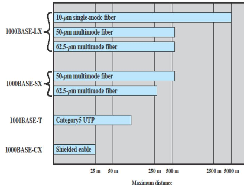
Figure 16.5 Gigabit Ethernet Medium Options (log scale)
