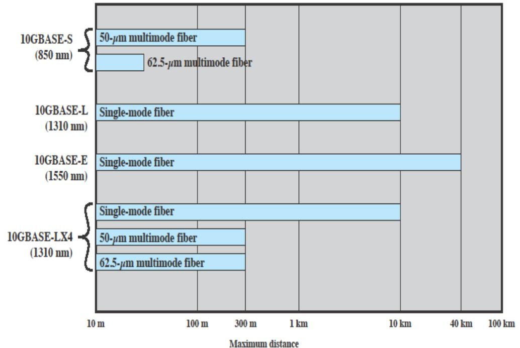
Figure 16.7 10-Gbps Ethernet Distance Options (log scale)
