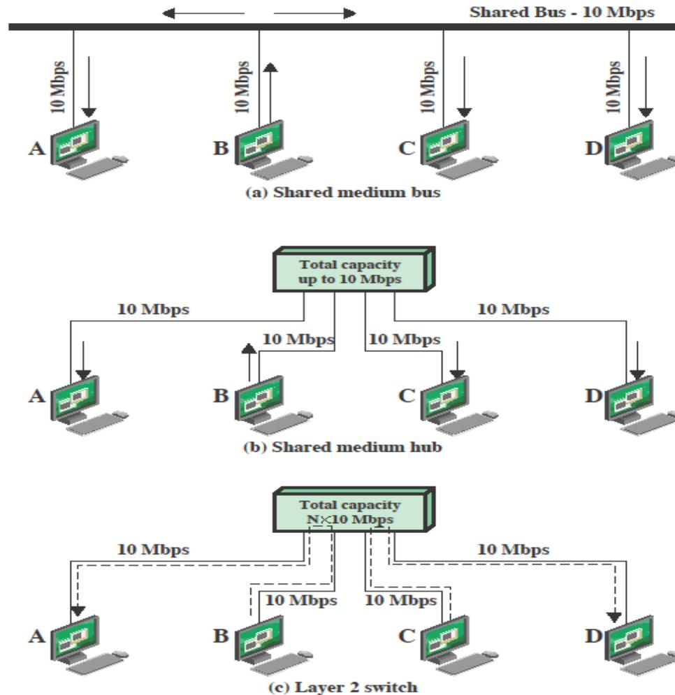
Figure 15.12 LAN Hubs and Switches
