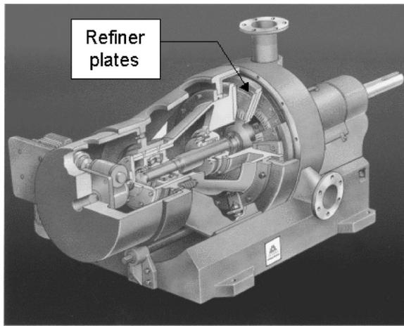
Fig. 4 A Low-Consistency Twin-Flo Disk Refiner
