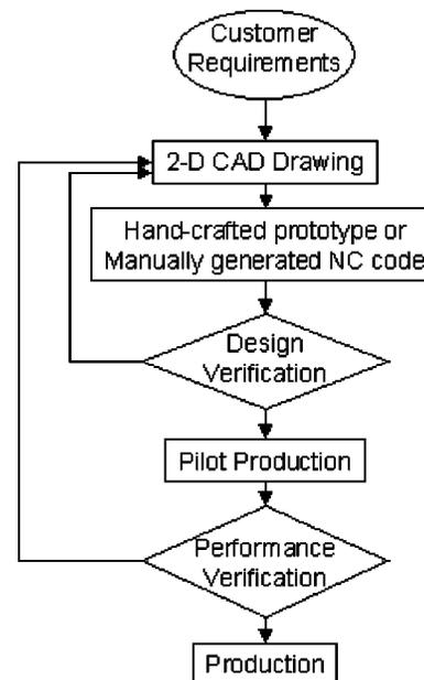
Fig. 2 Traditional Approach to Refiner Plate Design and Production [73]
