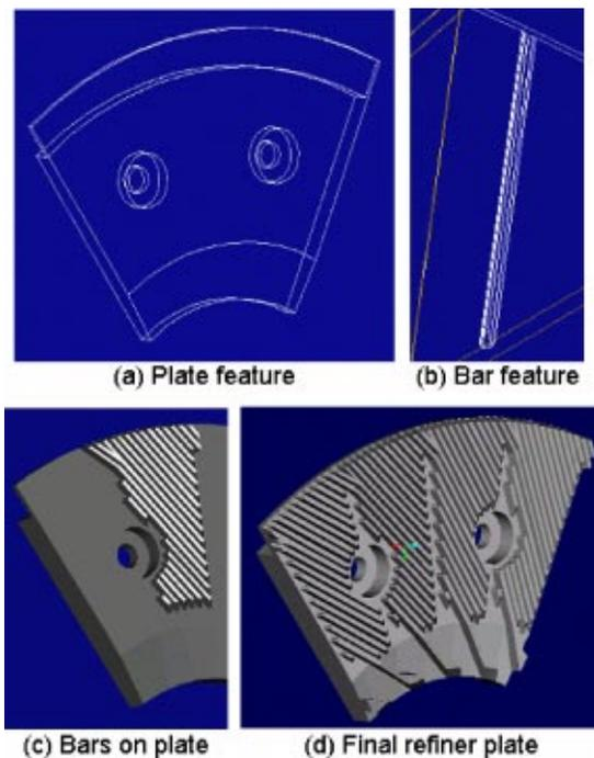
Fig. 6 Refiner Plate Model Generation in Pro/E
