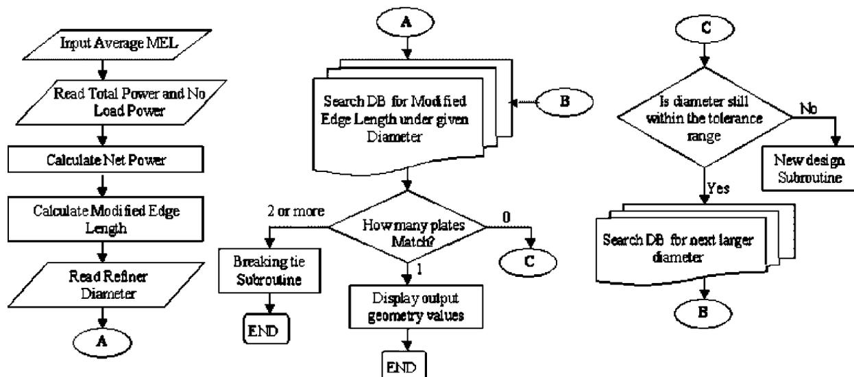
Fig. 5 Flowchart for Customizing a Refiner Plate
