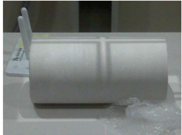
Figure 2. Plaster of Paris test specimen
