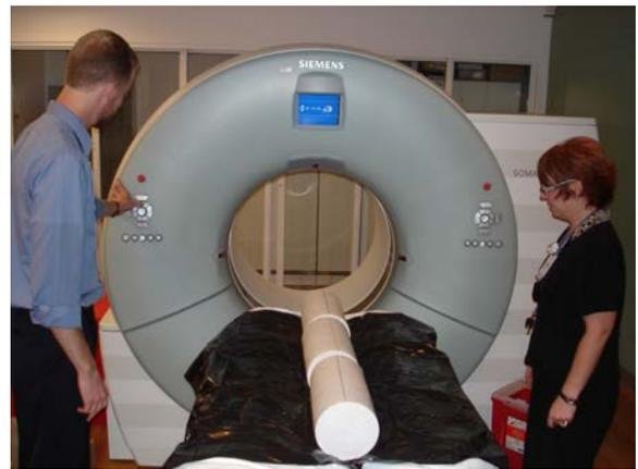
Figure 3. CT scanning of plaster specimen
